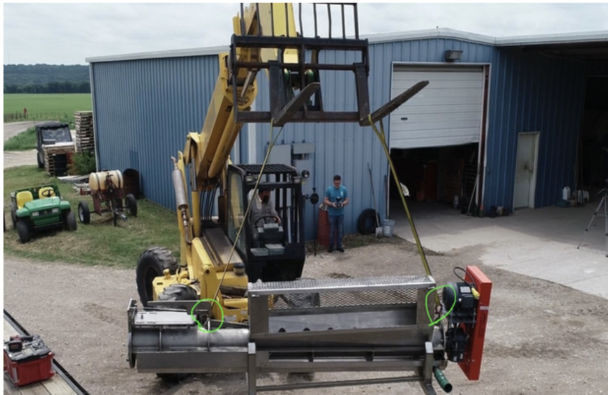
Pre-engineered lifting holes, circled in green, on the auger assembly. Attach shackles and straps here.
