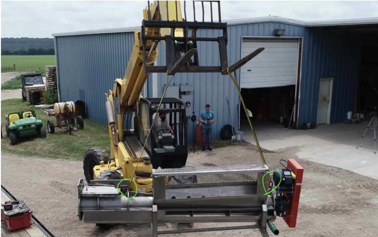
Auger assembly showing the two pre-engineered pick points (circled in green) — attach shackles and straps here
