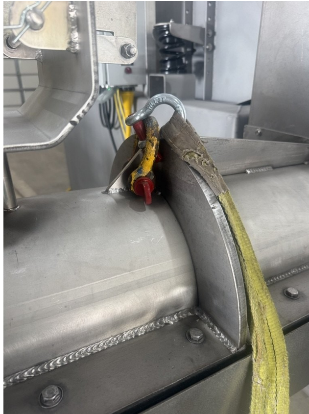
Lifting strap and bow shackle rigged at the auger assembly pick point.
