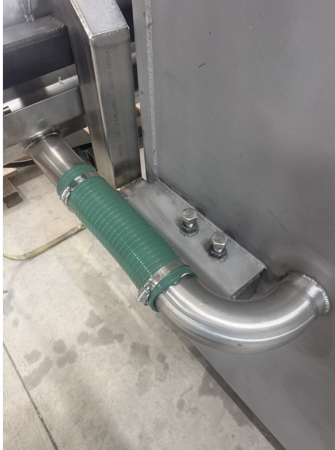
Auger drain-back connection from the drip pan to the capture tank, secured with two hose clamps. Note the auger mounting drawbar seated flush with the end of the receiver tube.
