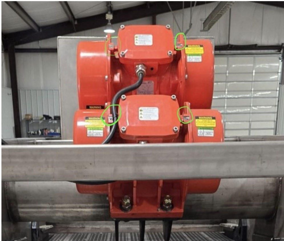
Grease points (circled in green) — two zerk fittings per motor, four total
