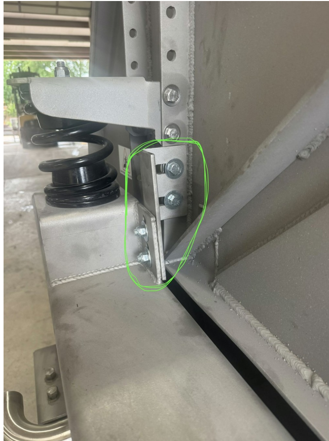
One of the four travel locks, located at each spring mount, securing the shaker basket for transit.
