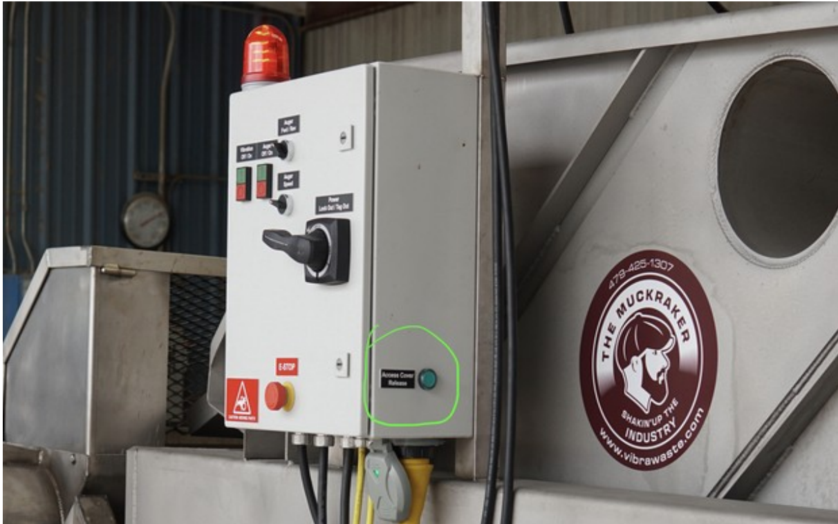
Earlier models: push-button Access Cover Release (circled in green). This version required two people, one to hold the button and one to open the hood.
