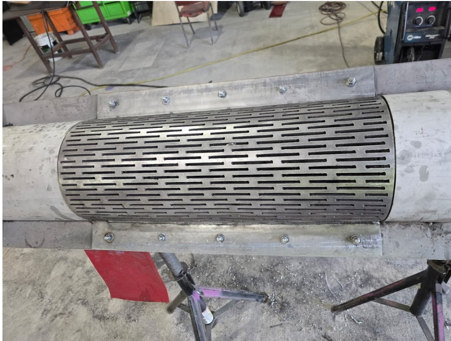
Underside of the extruder tube. Loosen the bolts shown to remove this section for cleaning. The catch pan must be removed first to access this area.
