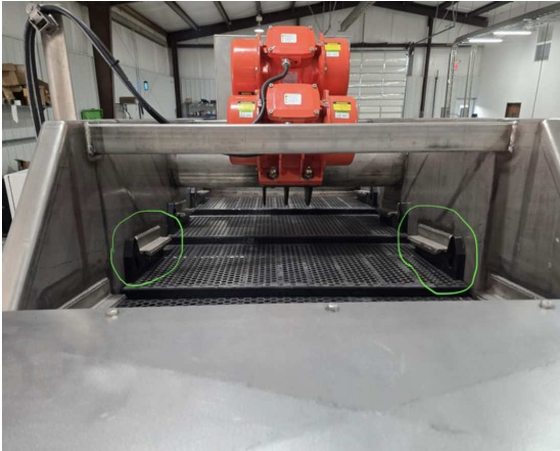
Wedge blocks in position (circled) securing screen elements in the shaker basket
