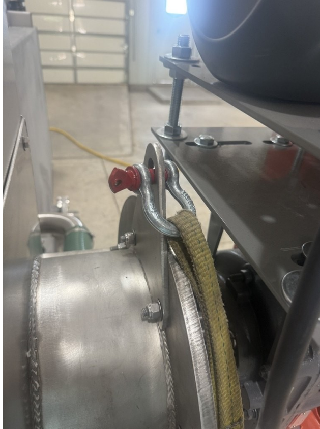
Bow shackle installed through a pre-engineered lifting hole with the lifting strap attached.
